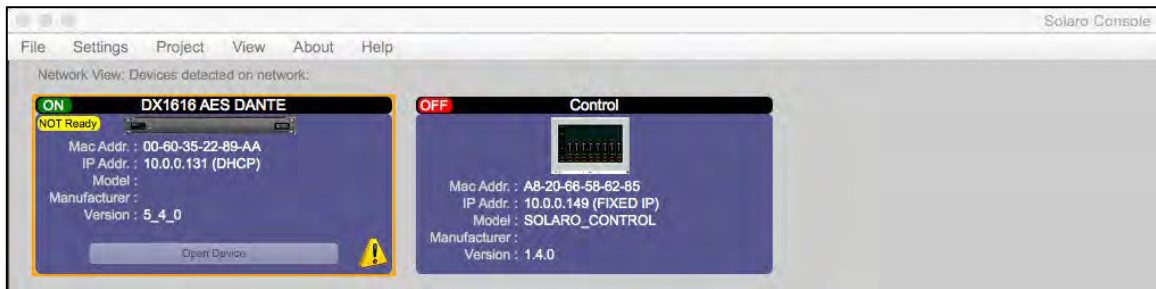
Figure 9: Firmware update – device not ready is shown
