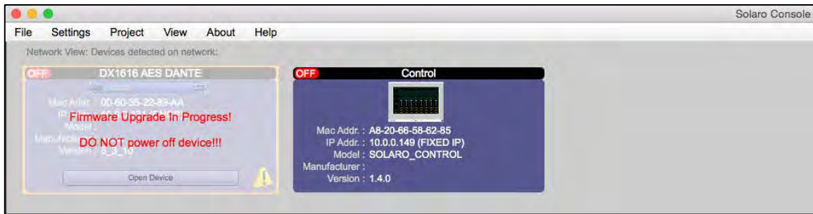
Figure 8: Firmware update in process – Do not power off the device
