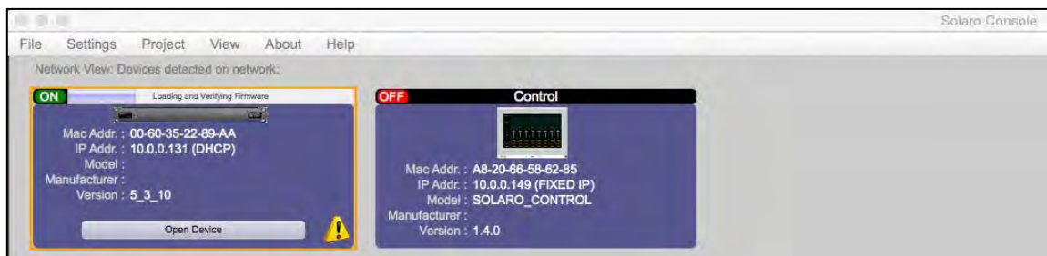
Figure 7: Firmware update in process – Loading and verifying firmware
